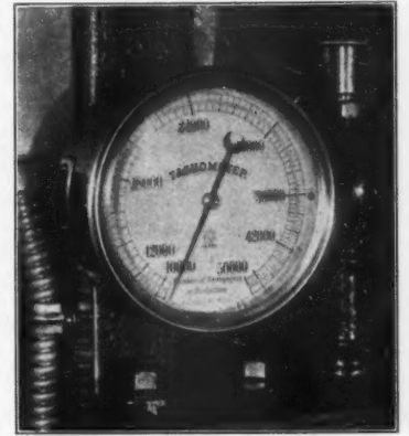
The tachometer showing the production speed of a press in number of papers per hour.
